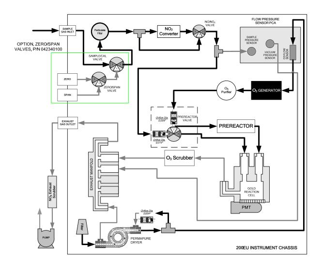
Figure 3-1: Pneumatic Diagram With Zero/Span Option
